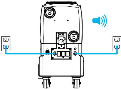
Each power cord on the Air Hog™ requires a grounded 15 amp outlet. The dual circuit indicator light and tone will activate when this is achieved. ♦
