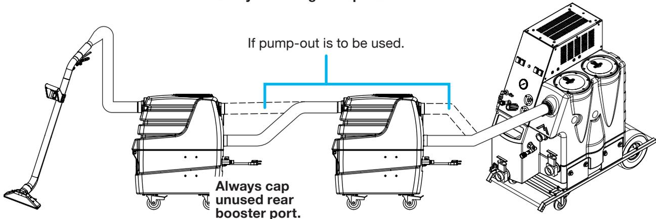
If the pump-out will be used, connect vacuum hose from extractor to top rear booster port and cap the bottom one. If not, connect hose to the bottom rear booster port and cap the top one. Recovered water will flow through the Air Hog™ to the extractor.
