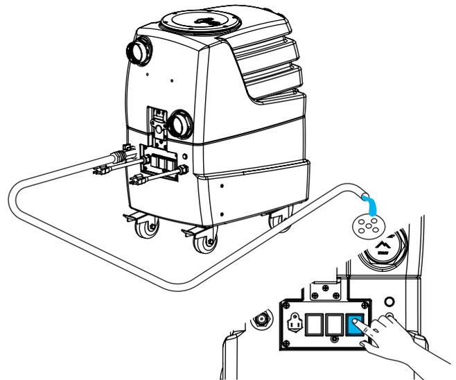
The recovery tank can be emptied using the pump-out feature. Attach a garden hose to the pump-out fitting, place the other end of the hose in a drain or receptacle, and press the PUMP-OUT switch on the switchplate. ♦
