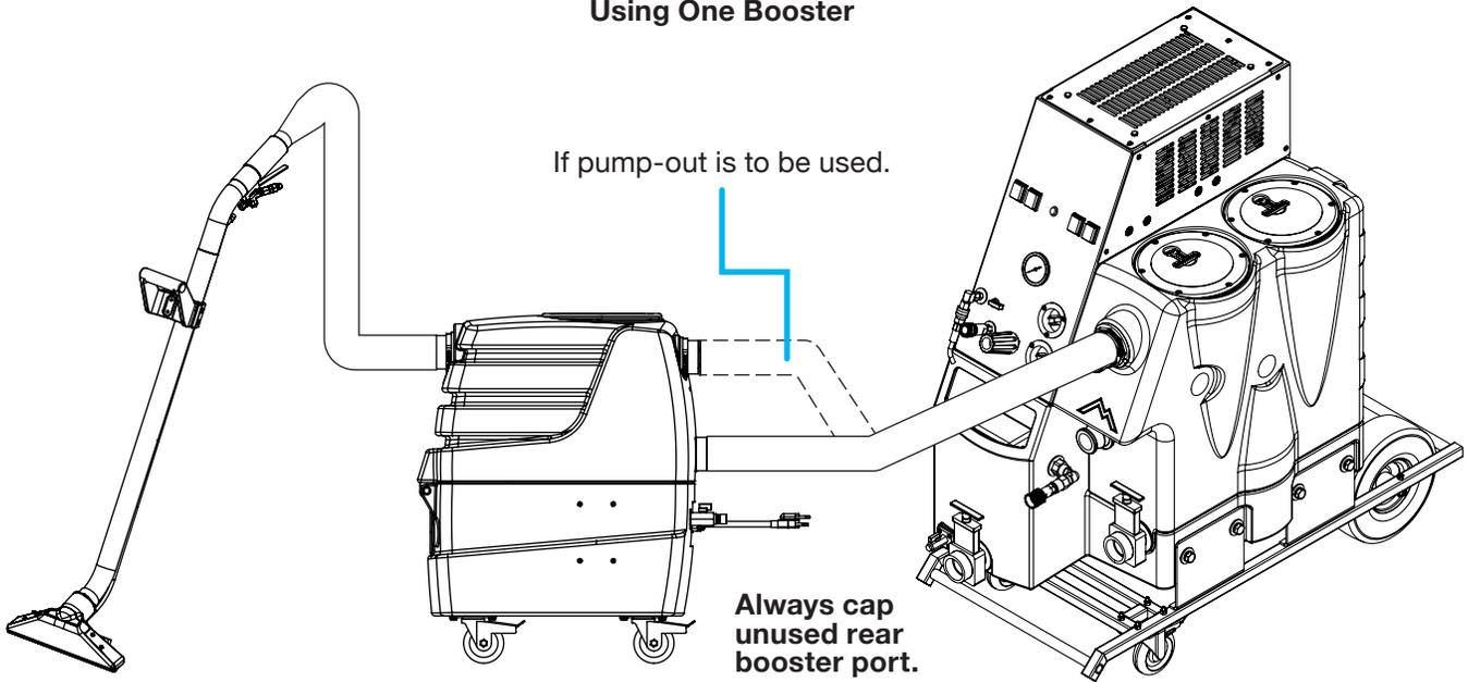
If the pump-out will be used, connect vacuum hose from extractor to top rear booster port and cap the bottom one. If not, connect hose to the bottom rear booster port and cap the top one. Recovered water will flow through the Air Hog™ to the extractor.
