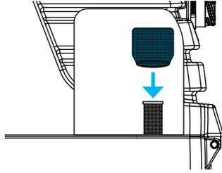
Use the included H141V or H110V female Cuff-Lynx™ Hose Connectors to connect 1.5" or 2" vacuum hose to the Cuff-Lynx™ starter on the front of the Air Hog™. The included H136V male Cuff-Lynx™ Connector can be used to connect 2" vacuum hose to either rear booster port. To attach a garden hose for use with the pump-out, thread the included garden hose quick connect onto the garden hose. The hose can then easily snap onto the Air Hog's™ pump-out fitting. ♦
